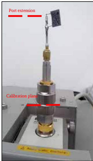
Measuring 0.1 Ohm SMD resistor for validation.
