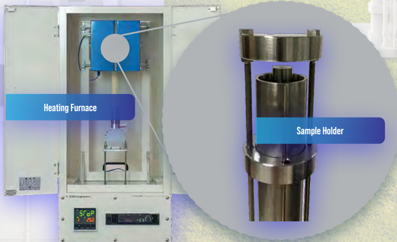
Heating Furnace and Sample Holder for HT-Z2-HF
