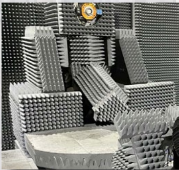
Figure 9: Low-scattering High-precision Positioner
